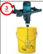
Continue to mix using a paddle drill and mortar mixing paddle for an additional 3 minutes or until components are thoroughly blended.
