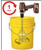
Mix A & B Components using drill at slow speed for 1 minute (if using optional pigment pack to pigment urethane cement add 8 oz of pigment to 2 gal mix.
