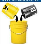
Pour A-Components and B-Components at mix ratio of 1A:1B into a clean 5-gallon metal bucket.
